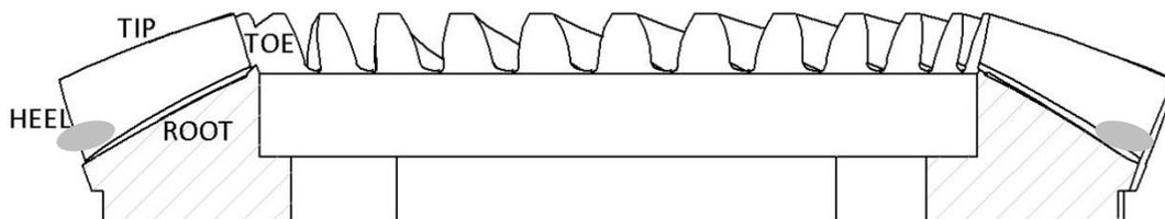
Contact further to heel and tip than factory marking.
