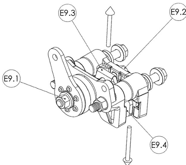
1. Remove the Nut (E9.1) and slide the Bolt (E9.2) out through the Calliper body.
