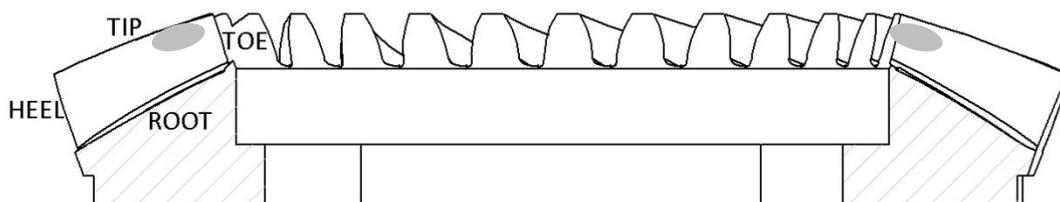
Contact further to toe and tip than factory marking.
