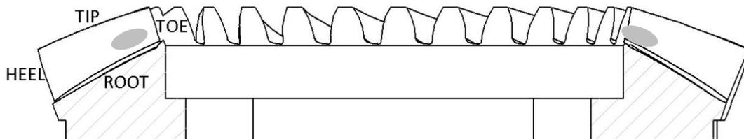
Contact further to toe and root than factory marking.
