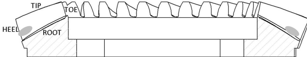
Contact further to heel and root rather than factory marking.
